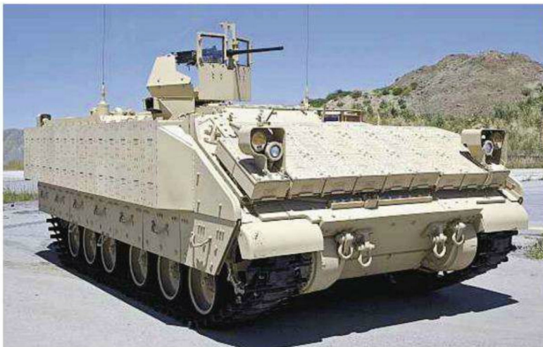
A Bradley Mortar Vehicle with a 120 mm mortar and fitted with a roof-mounted protected weapon station armed with a .50 cal M2 HB machine gun. This example is also fitted with ERA.
